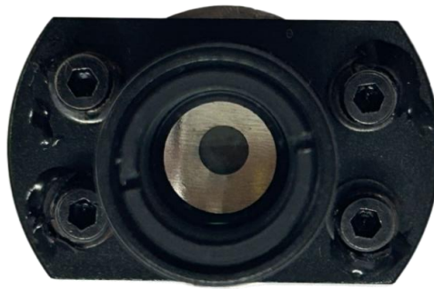
Fig. 3. The front schematic of the proposed varifocal Alvarez lenses, where the four screws are used for assembly with the drive structure.
